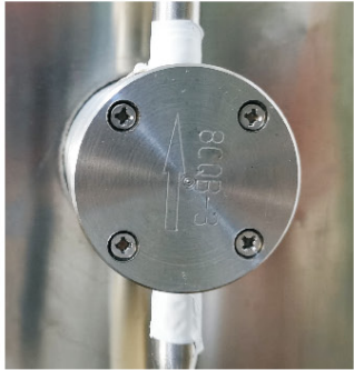
磁力泵 Magnetic Gear Pump
